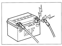
Before measuring voltage at each terminal, check to make sure that battery voltage is 11 V or higher. Terminal voltage check at low battery voltage will lead to erroneous diagnosis.
