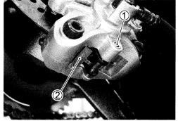
• Remove the brake pads.
