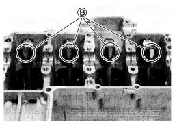
Apply MOLYBDENUM OIL SOLUTION to the crank pin bearings surface.
