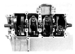
Apply MOLYBDENUM OIL SOLUTION to the crank pin and bearing surface.
