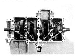
• Insert the right and left-thrust bearings with oil groove ® facing the crank web.
