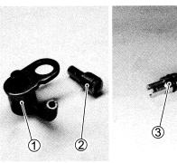
• Fit the new O-rings ① to each piston cooling oil jets as shown and apply engine oil to them.
