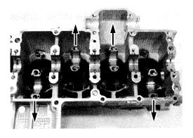
• Set the crankshaft to the conrods and upper crankcase.
