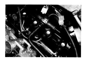
The valve clearance specification is different for intake and exhaust valves. Valve clearance must be checked and adjusted, 1) at the time of periodic inspection, 2) when the valve mechanism is serviced, and 3) when the camshafts are removed for servicing.
