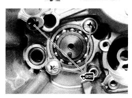
• Remove the piston cooling oil jets ① from the upper crank-case.
