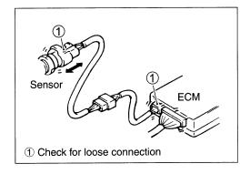
Using a test male terminal, check the female terminals of the circuit being checked for contact tension.
