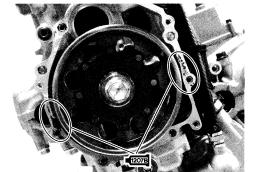
Install the dowel pins ① and new gasket ②.
