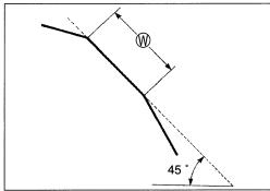
If the valve seat is pitted or burned, use the 45 ° cutter to condition the seat some more.
