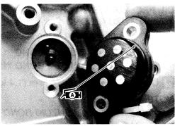
• Install the gear position switch ③ as shown.
