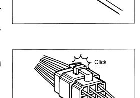
Inspect each lead wire circuit for poor connection by shaking it by hand lightly. If any abnormal condition is found, repair or replace.
