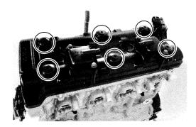
• Remove the dowel pins and O-rings.
