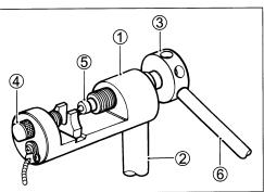
• Stake the joint pin by turning (approximately 7/8 turn) the pressure bolt "A" ③ with the bar until the pin end diameter becomes the specified dimension.
