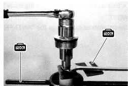
• Remove the spacer ⑥, spring retainer ⑤, spring ⑦, adjuster rod ⑧ and front fork cap ⑨.
