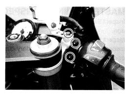
• Remove the reservoir cap ①, insulator ② and diaphragm ③.
