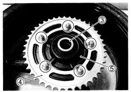
• Remove the rear sprocket mounting drum retainer 6.
