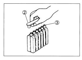
Insert the nozzles of the electrolyte container into the battery's electrolyte filler holes, holding the container firmly so that it does not fall. Take precaution not to allow any of the fluid to spill.
