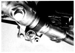
• Remove the radiator mounting bracket ① and the oil cooler mounting bracket ②.
