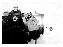
Remove the STP sensor 9 with the special tool.
