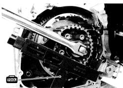
• Remove the concaved washer ④, washer ⑤, clutch sleeve hub ⑥ and washer ⑦.
