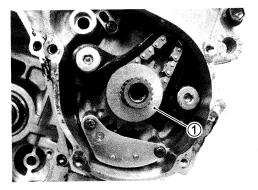
Install the starter clutch assembly onto the crankshaft.
