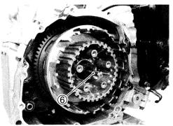
• Unlock the clutch sleeve hub nut.
