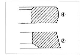
• 1st ring and 2nd ring have letters "R" and "RN" marked on the side. Be sure to bring the marked side to the top when fitting them to the piston.
