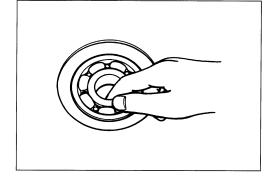
Remove the wheel bearings with the special tool.
