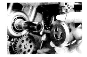
• Install the oil pump drive gear ① to the primary driven gear assembly.
