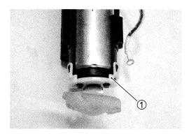
· Remove the fuel mesh filter.
