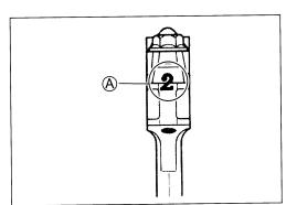
• Check the corresponding crank pin O.D. code number ("1", "2" or "3") (B).
