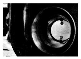
5) Turn the ignition switch ON to check the STVA operation. (STV operating order: Full open  $\rightarrow$  95 % open)
