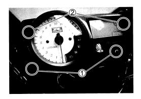
• Disassemble the combination meter as follows.
