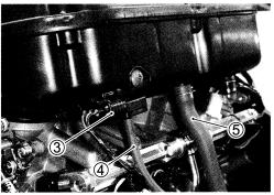
• Loosen the throttle body clamp screws.
