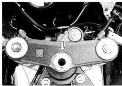
· Draw out the handlebars to upward.
