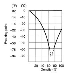
Fig.1 Engine coolant density-freezing point curve.
