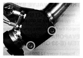
• Check the lock-nuts tightness. If the lock-nuts are loose, adjust the cable play and tighten the lock-nuts.
