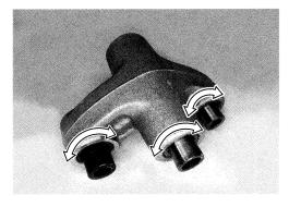
• Draw out the cushion lever bearings with the special tool.
