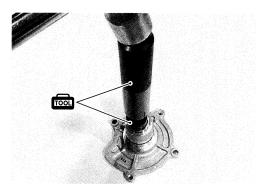
• Apply SUZUKI SUPER GREASE to the impeller shaft.
