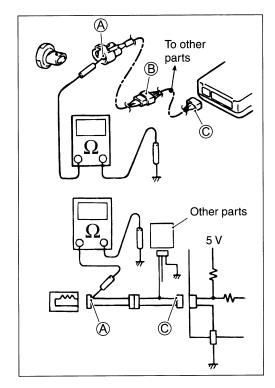
Disconnect the connector/coupler included in circuit (coupler
