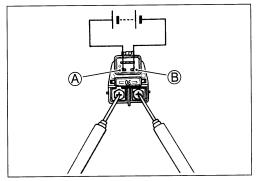
Measure the relay coil resistance between the terminals using the multi circuit tester. If the resistance is not within the specified value, replace the starter relay with a new one.
