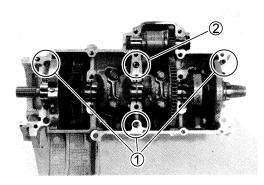
Apply SUZUKI BOND to the mating surface of the middle crankcase.
