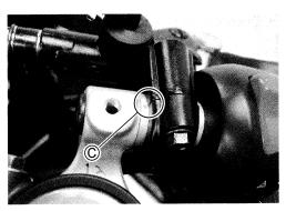
Apply the SUZUKI SUPER GREASE to the throttle cables and their holder.
