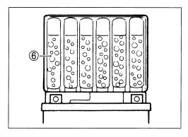
If no air bubbles are coming up from a filler port, tap the bottom of the electrolyte container two or three times.
