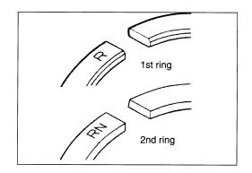
Position the gaps of the three ring as shown. Before inserting each piston into the cylinder, check that the gaps are so located.
