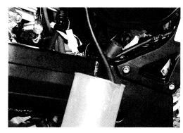
• Apply 12 volts to the fuel pump for 30 seconds and measure the amount of fuel discharged.
