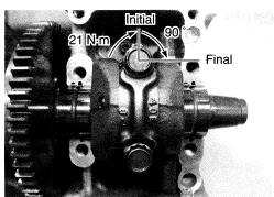
Apply MOLYBDENUM OIL SOLUTION to each crankshaft journal bearing lightly.
