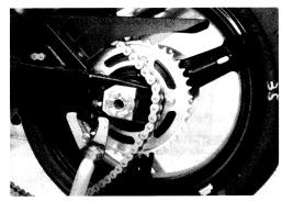
• Remove the engine sprocket ⑤.
