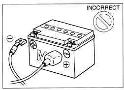
Removing any battery terminal of a running engine is strictly prohibited.
