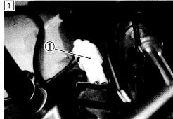
4) Disconnect the CKP sensor coupler ① and measure the resistance.
