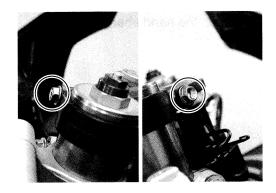
• When remounting the clutch lever holder, align the holder's mating surface (A) with punch mark (B) on the handlebar.
