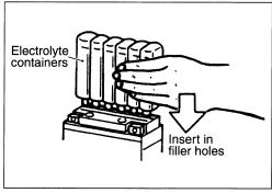
Make sure air bubbles 6 are coming up each electrolyte container, and leave in this position for about more than 20 minutes.
