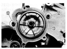
Install the starter idle gear cover and tighten its bolts to the specified torque.
