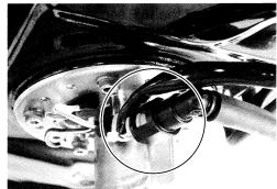
• Disconnect the vacuum hose ① from the PAIR valve.
