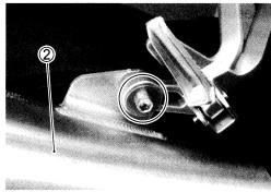
• Remove the EXCV cover 3 and disconnect the two cables from the EXCV pulley.
