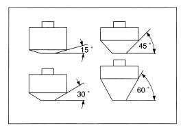
• When installing the solid pilot ①, rotate it slightly. Seat the pilot snugly. Install the 45 ° cutter, attachment and T-handle.
