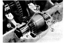
• Set the balancershaft so that its punch mark A is aligned with the index B on crankshaft.
