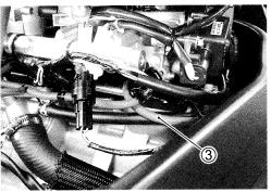
• Connect one of the vacuum balancer gauge hose 4 to the nipple on the No.4 throttle body.
