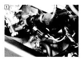
4) Disconnect the injector coupler and measure the resistance between terminals.
