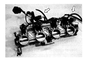
• Disconnect the respective vacuum hoses ① and EVAP purge hoses ② from each throttle body. (For E-33)
