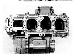
Remove the lower crankcase and measure the width of the compressed plastigauge using the envelope scale. This measurement should be taken at the widest part of the compressed plastigauge.
