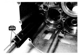
• Remove the gearshift cam bearing with the special tools.
