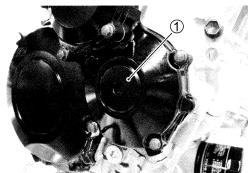
• Turn the crankshaft to bring the line (A) on the starter clutch to the index mark (B) of the valve timing inspection hole and also to bring the cams to the position as shown.
