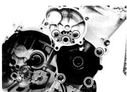
• Remove the wave washer ④, the starter idle gear No.2, ⑤ and its shaft ⑥.
