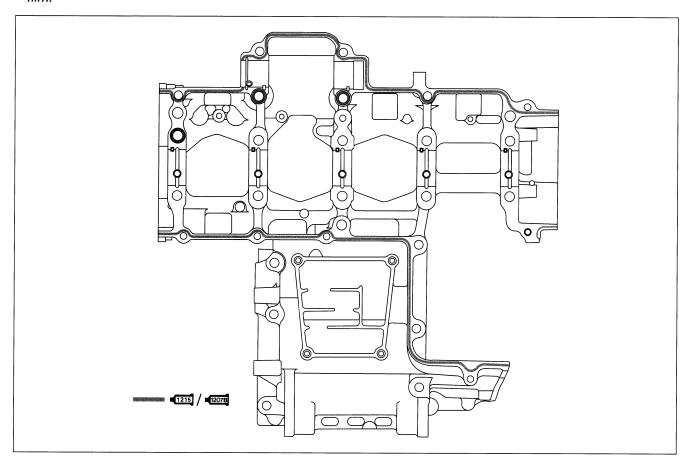
• Tighten the crankcase bolt (9 mm) in ascending order of numbers assigned to these bolts. Tighten each bolt a little at a time to equalize the pressure in the following two steps.
