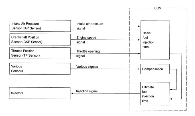
The following different signals are output from the respective sensors for compensation of the fuel injection time (volume).
