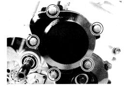
• Remove the shaft ①, washer ②, starter idle gear No.1 ③, concaved washer, bearing and washer.
