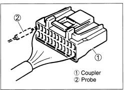
When connecting meter probe from the terminal side of the coupler (connection from harness side not being possible), use extra care not to force and cause the male terminal to bend or the female terminal to open.
