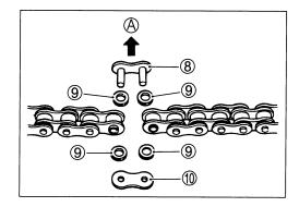
Apply grease on the recessed portion of the joint plate holder
