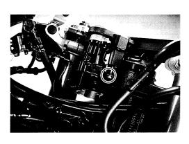
Inspect each switch for continuity with a tester. If any **STARTER BUTTON** abnormality is found, replace the respective switch assemblies with new ones.
