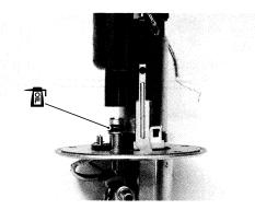
• Pass through the wires behind the thermistor ①.
