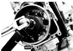
• Install a bolt (A) of suitable size to the left end of crankshaft.
