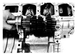
• Install the driveshaft assembly on the upper crankcase.
