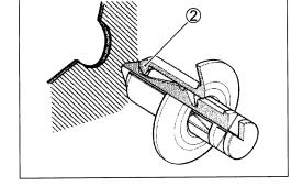
• Push in the head of center piece until it becomes flush with the fastener outside face.
