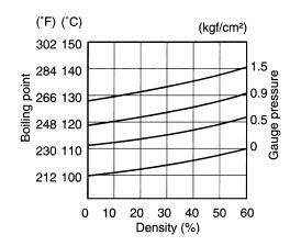
Fig.2 Engine coolant density-boiling point curve.
