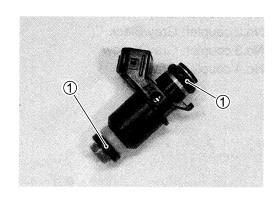
• Apply thin coat of the engine oil to the new O-rings ②.
