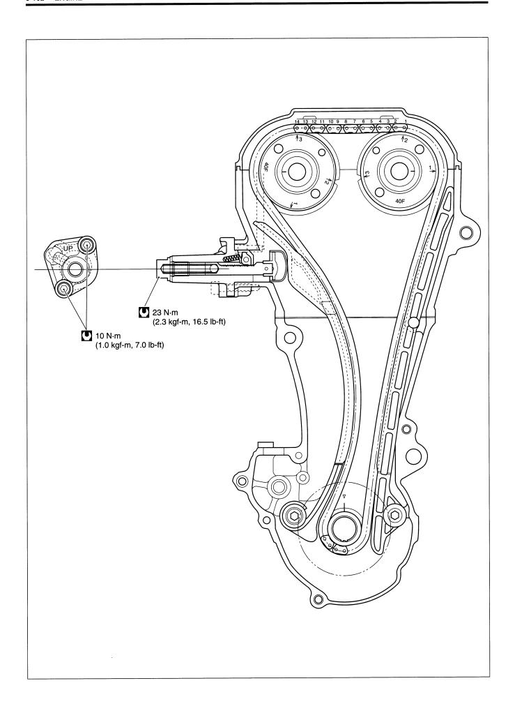
• Tighten the valve timing inspection plug 7 to the specified torque.
