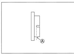
• The extent of brake pad wear can be checked by observing the grooved limit line (A) on the pad. When the wear exceeds the grooved limit line, replace the pads with new ones. ((3)8-65)
