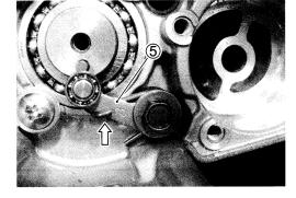
• Install the gearshift cam stopper plate after aligning the gearshift cam pin A with the gearshift cam stopper plate hole B.
