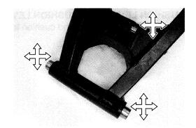
• Draw out the swingarm pivot bearings ① and the swingarm cushion rod upper bearings ② with the special tool.
