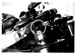
Place a rag underneath the union bolt on the master cylinder to catch any split brake fluid. Remove the union bolt and disconnect the brake hose.
