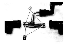
• Assemble the fuel delivery pipes.
