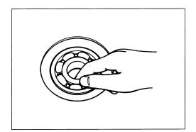
• Remove the sprocket mounting drum bearing and wheel bearings with the special tool.
