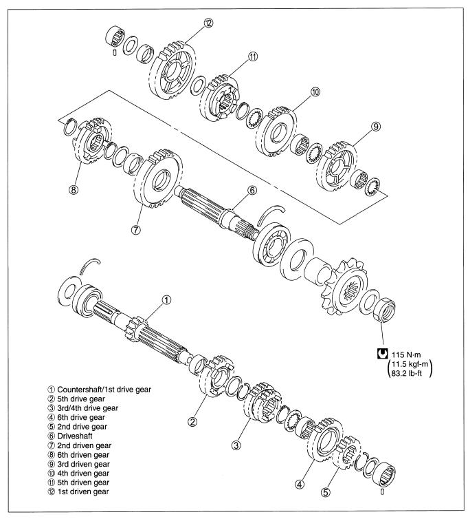
Assemble the countershaft and driveshaft in the reverse order of disassembly. Pay attention to the following points:
