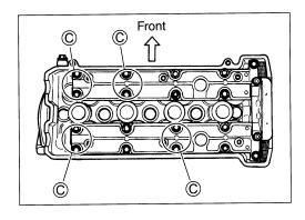
The clearance is adjusted by replacing the existing tappet shim by a thicker or thinner shim.
