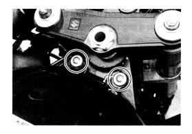
• Lift and support the fuel tank with the fuel tank prop stay ①.
