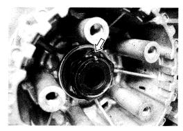
• Hold the clutch sleeve hub with the special tool.
