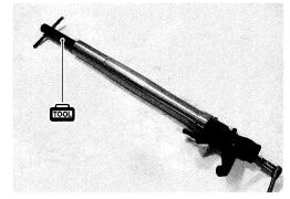
• Remove the inner rod/damper rod (cartridge) 10.
