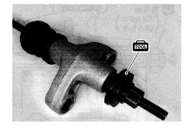
Apply SUZUKI SUPER GREASE to the bearings, spacers, washers and dust seals.
