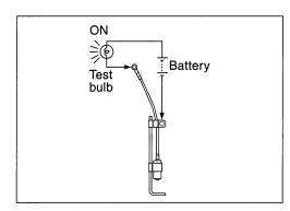
When the switch is immersed in water under the above condition, the bulb should go out. If the bulb remains lit, replace the unit with a new one.
