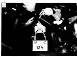
4) Then, swap the wires supplied 12 volts and check the operation of EXCVA.(Check the operation of EXCVA both way)
