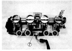
• Remove the TP sensor ® with the special tool.
