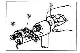
• Turn in the pressure bolt "B" 4 with the bar 5 and force out the drive chain joint pin 9.
