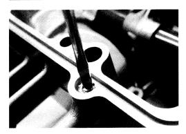
Remove the oil jet ② (for cam chain tension adjuster) from the cylinder head.
