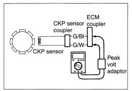
If the peak voltage is lower than the standard range, check the peak voltage at the CKP sensor lead wire coupler.
