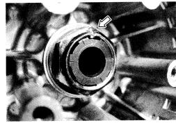
• Install the spring washer seat ® and spring washer 9 onto the clutch sleeve hub correctly.
