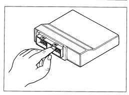
When disconnecting and connecting the ECM, make sure to turn OFF the ignition switch, or electronic parts may get damaged.
