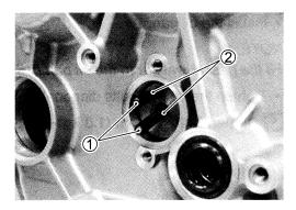
• Apply the SUZUKI SUPER GREASE to the O-ring.
