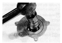
• Install the new bearings with the special tool.
