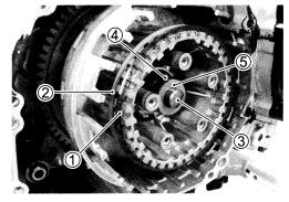
• Remove the clutch push rod 6.
