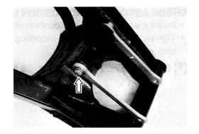
• Remount the chain case 1 and chain buffer 2.
