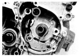
Apply SUZUKI BOND light to the groove of the signal generator lead wire gromet.
