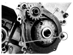
• Install the starter clutch cover and tighten its bolt as shown.
