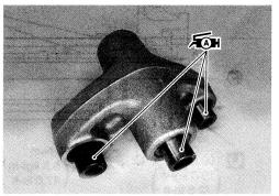
Assemble the cushion rod onto the swingarm temporarily.
