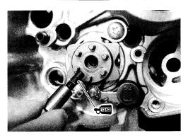
• Install the gearshift shaft/gearshift arm 6 with the washers as shown.
